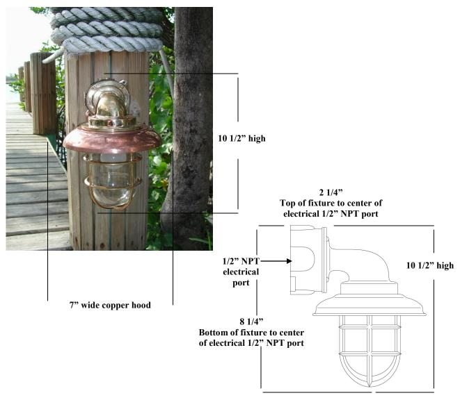
Medium 90 degree heavy solid <u>Bronze</u> Passageway ship's light! This light weighs approximately 9 pounds and was used to light up ship's hallways. The heavy bronze lights have a heavy bronze cage that spins off and the extra thick glass globe also spins off to access the light bulb. The light is approx 10 1/2" high and 7" wide (copper ring) and 9 1/4" deep. Copper trim ring is included.
